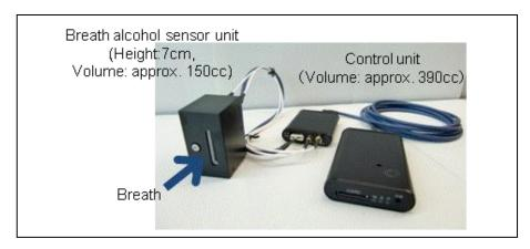
Prototype breath alcohol detection system
