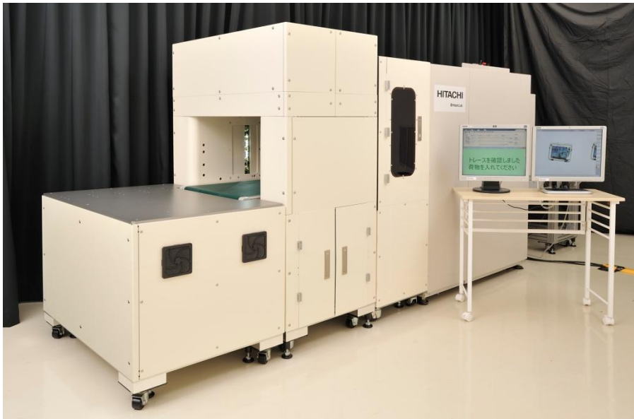
Prototype explosives detection system for carry-on luggage (Courtesy of Hitachi Power Solutions Co., Ltd.)
