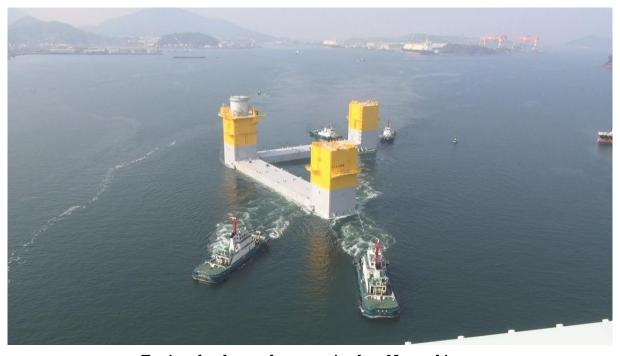
Towing the three-column semi-sub at Nagasaki port
