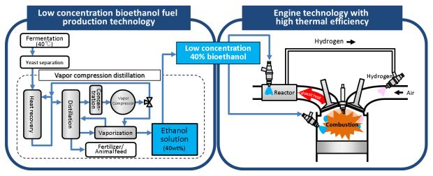
Fig. 1 A flow from producing the low concentration bioethanol fuel to power generation
