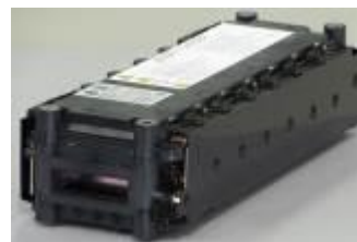
A lithium-ion battery module
