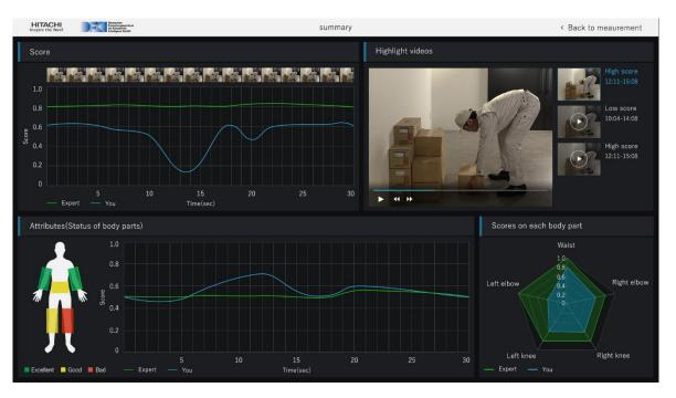
Test screen showing real-time measurement and comparison/assessment of differences with the model worker Changes in physical load evaluation with time (upper left) Video of an improper movement (upper right) Changes in the status of body parts with time (lower left) Evaluation of each body part (lower right)
