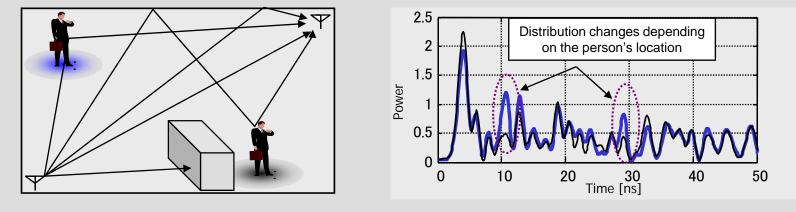
Fig 1. Receiving reflected waves
