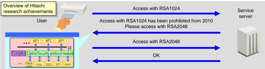
Automatically customize the protocol within the IC card to RSA2048
