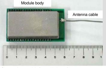
GPS transmitter module for use indoors (60 × 30-mm prototype)
