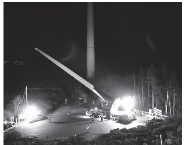
Figure 3 — Blade Lifter in Action Transporting Blade
