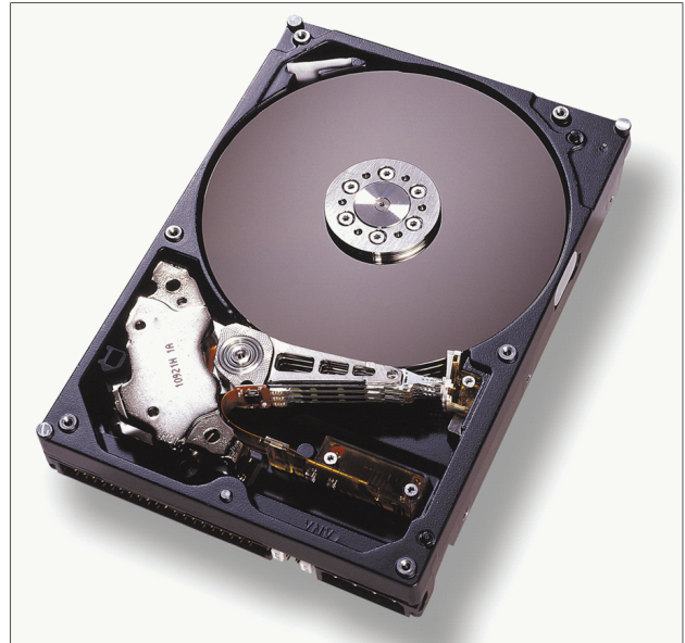
Fig. 7—Hitachi Global Storage Technologies, Inc.'s HDD. The 120-Gbyte HDD used in the new digital recorder. Achieves high-speed reading performance by spinning a 3.5 inch disk at 7,200 rpm.
