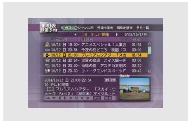
Fig. 4—EPG Channel by Channel Display. By periodically receiving broadcast data on TV programs, a variety of applications can be displayed. This screen shows the information for a particular channel.
