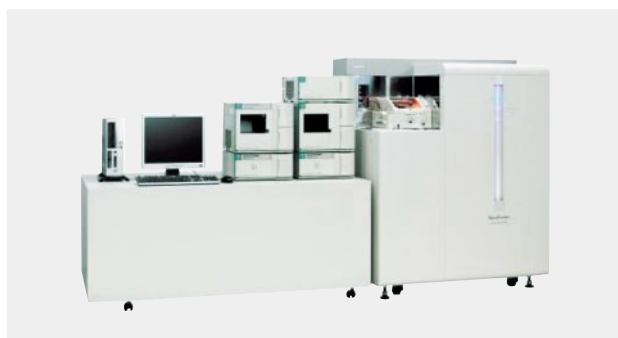
Fig. 1—NanoFrontier Exterior. The control computer and the nanoLC are on the left side and the trap-TOFMS is on the right side.
