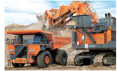
Ultra-large hydraulic excavator and rigid dump truck for mining
