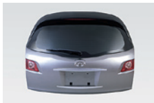
Hitachi Chemical's molded plastic rear hatch door
